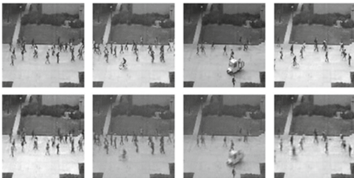
Fig. 4 Reconstruction of frames belonging to UCSD-PED2 dataset. Top row: original frames. Bottom row: reconstructed frames using R-STAE
